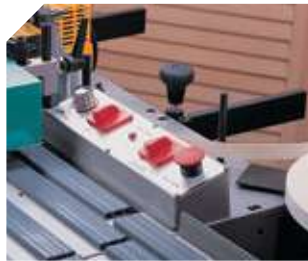
Safety control (STOP). Electronic temperature control.
