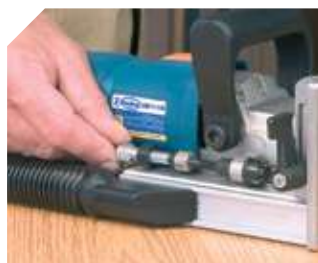
Quick adjustment of different slotting depths.
