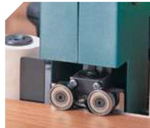
Power trimming unit: trimming both sides simultaneously.
