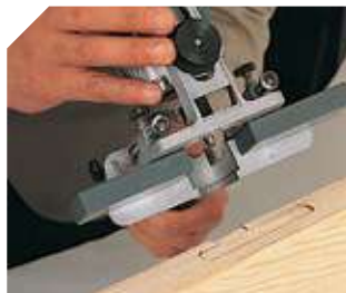
Placing hinges with the ZB93 head.
