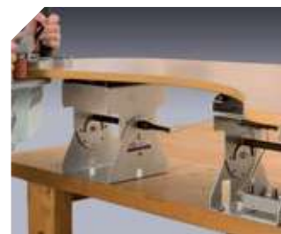
Gripping large pieces with the help of an SVN470 auxiliary unit.
