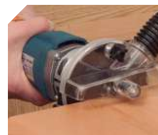
Round head (V3) included with the set. Very practical for trimming with support on edges and essential for jobs that require this type of work.
