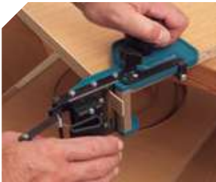
Cutting on both sides on straight panels.
