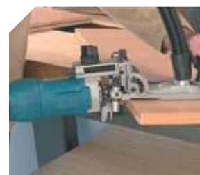
Trimming the edge with the straight bit.
