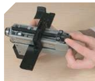
Micrometric regulation of the cutting width.
