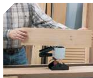
Gluing with the upper roller.
